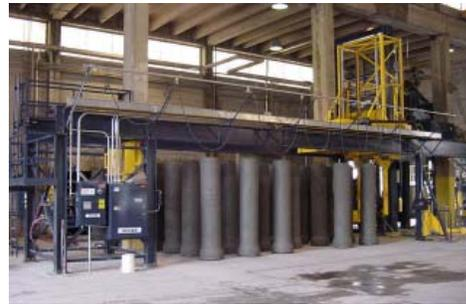
pipe forms on and off the pipe machine to the moving kiln floor. Start-up began immediately after Labor Day and full production was achieved within a few weeks.
